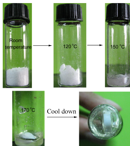
Fig. 2 Photographs of the appearance of Bisphenol-S mixing with MImBS
